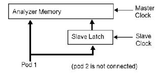
pod into the logic analyzer memory that is normally used for two pods.
